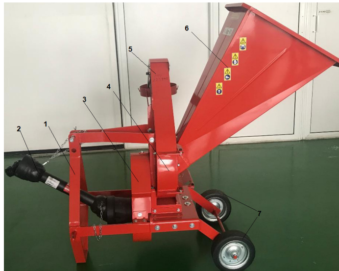
Fig. 3. BIO 90 grinder: 1 – frame, with 3 point hitch strut; 2 – universal joints transmission; 3 – belt transmission; 4 – grinding device; 5 – grinded material chute; 6 – feeding chute
