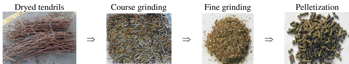
Fig. 1. Technological phases for pelletization of vine tendrils (natural drying)
